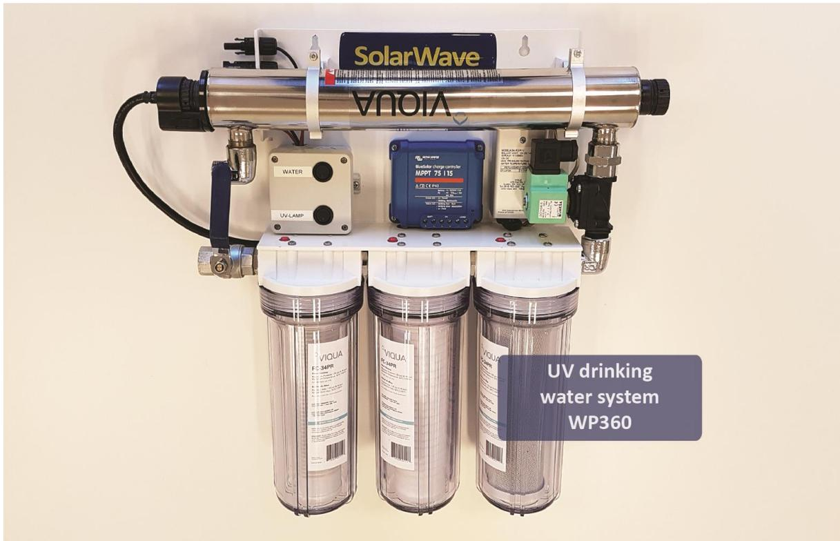
The *SolarWave WP360* is a solar powered water purification system that cleans water using proven ultra violet (UV) disinfection technology and fine sediment and carbon pre-filters. UV is a chemical free process which deactivates bacteria, virus, and protozoa by up to 99.99%, thus providing clean and safe drinking water which meets the World Health Organization's and local health departments' standards for potable water.
